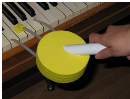
Figure 3: The chord-playing device made out of layered foam core and tubing.
