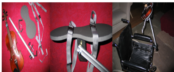
Figure 2: Height and angle adjustable violin tray attached with interlocking tubing to wheelchair.
